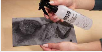
The rock forming mould is sprayed with a release agent consisting of water (20:1) and detergent.
