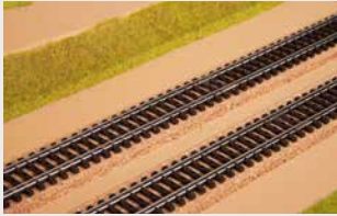
The rail is laid and fixed onto the cork track bed.
