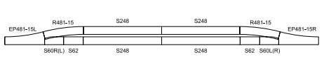
V4 Ref. 7078634, Variation Set V4 / KATO 20-863, Switching Siding Set Create a station or signal point to allow trains to overtake.
